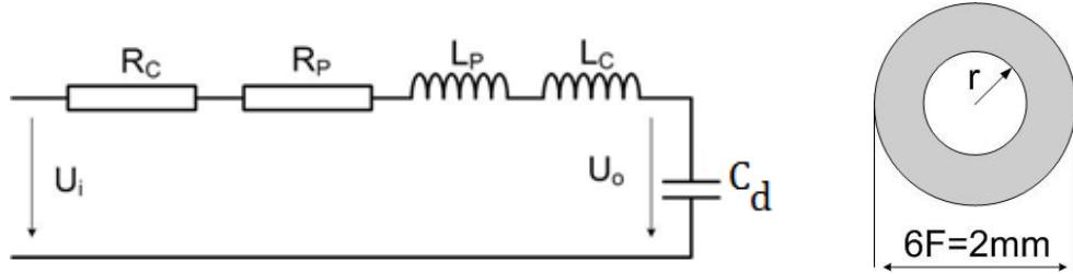
External diameter of catheter<sup>1</sup> = 6 F, or equivalently, 2 mm
